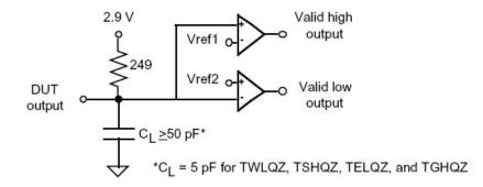
**Tester Equivalent Load Circuit**
